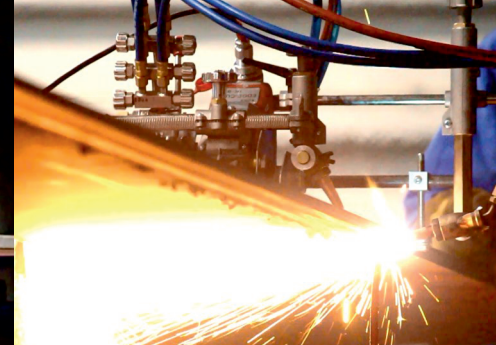
Chamfering (1 :4 ratio bevelling) using single torch
