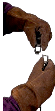
Chain links can be adjusted easily for various pipe diameters.
